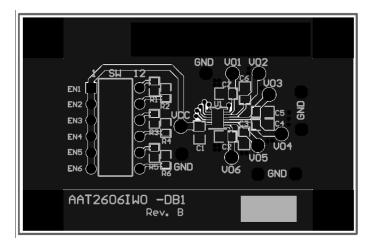
Figure 2: AAT2606 Evaluation Board Top Side Layout.
