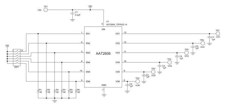
Figure 1: AAT2606 Evaluation Board Schematic.
