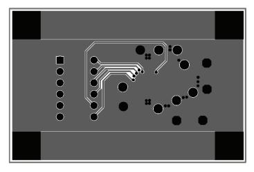
Figure 3: AAT2606 Evaluation Board Bottom Side Layout.
